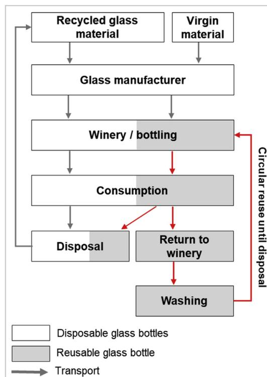
**Fig. 2.** Process flow diagram of single use and reusable glass bottles.
